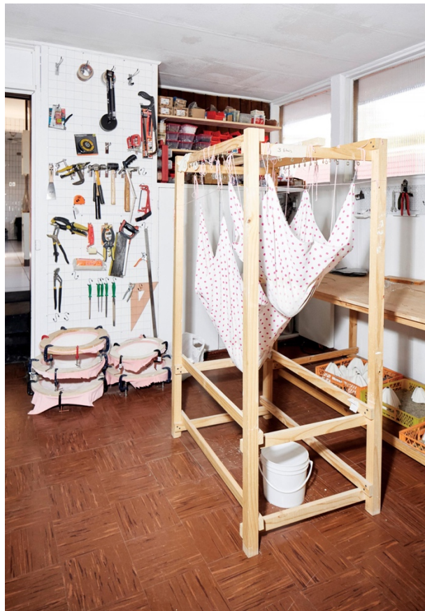
To produce Less CPP , Gt2p developed what it calls a 'catenary pottery printer'; its wooden framework supports draped fabrics that filter ceramic slip for the fabrication of moulded forms.
