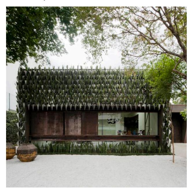
The faceted aluminium containers hang from a mounted wire grid on the exterior of the two-storey Firma Casa store.
