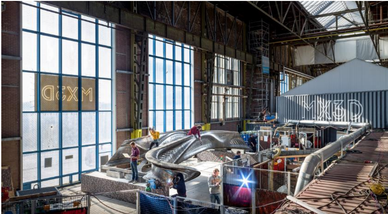
The MX3D bridge, which was 3D-printed by robotic arms, is one of Laarman's best-known projects. Photograph by Thijs Wolzak
