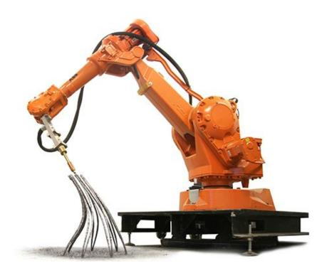
Joris Laarman's MX3D printer is a 3-D printing robot that can build objects using metals ranging from steel to copper. (Courtesy of Joris Laarman Lab)
