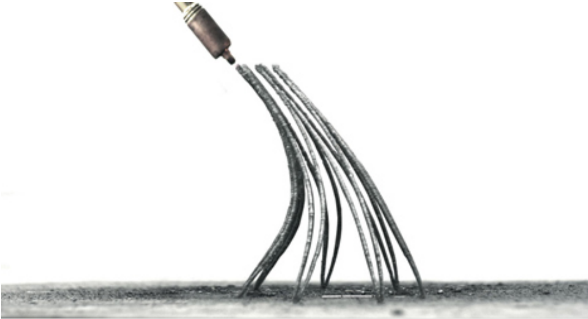
Robot arm 3D-printing metal lines
