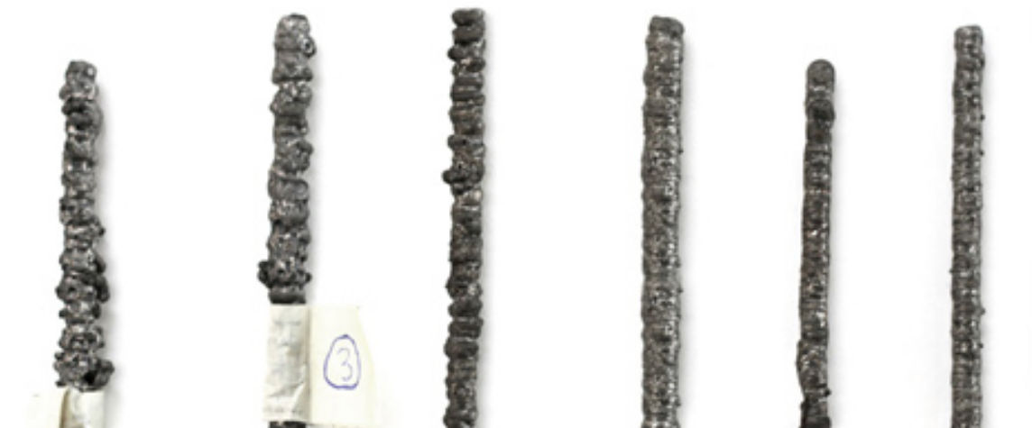
Examples of 3D-printed metal lines
