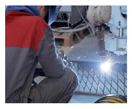
"The basics of the technology is pretty simple," Laarman explains in the movie, which was filmed at MX3D's workshop in Amsterdam. "We're using an industrial robot that is usually used in assembly lines in the car industry. We have combined this with a welding machine and our own software to have it 3D print in metal."
