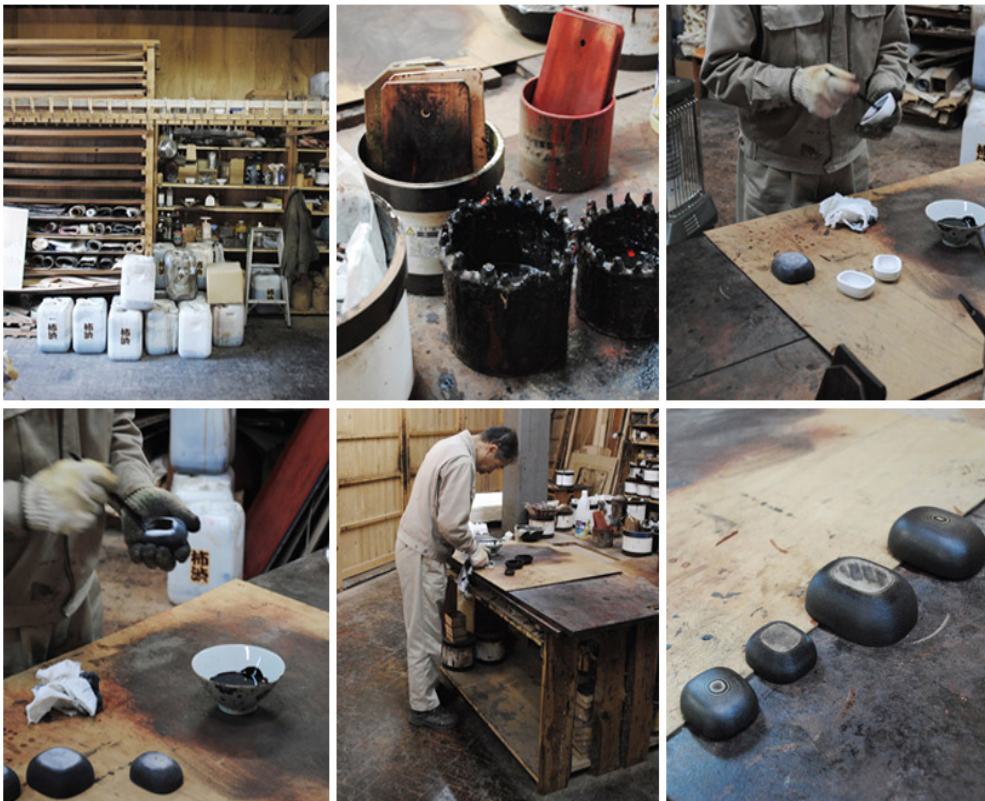
to complete the paper-constructed three dimensional objects, a layer of lacquer is applied to solidify the surface
